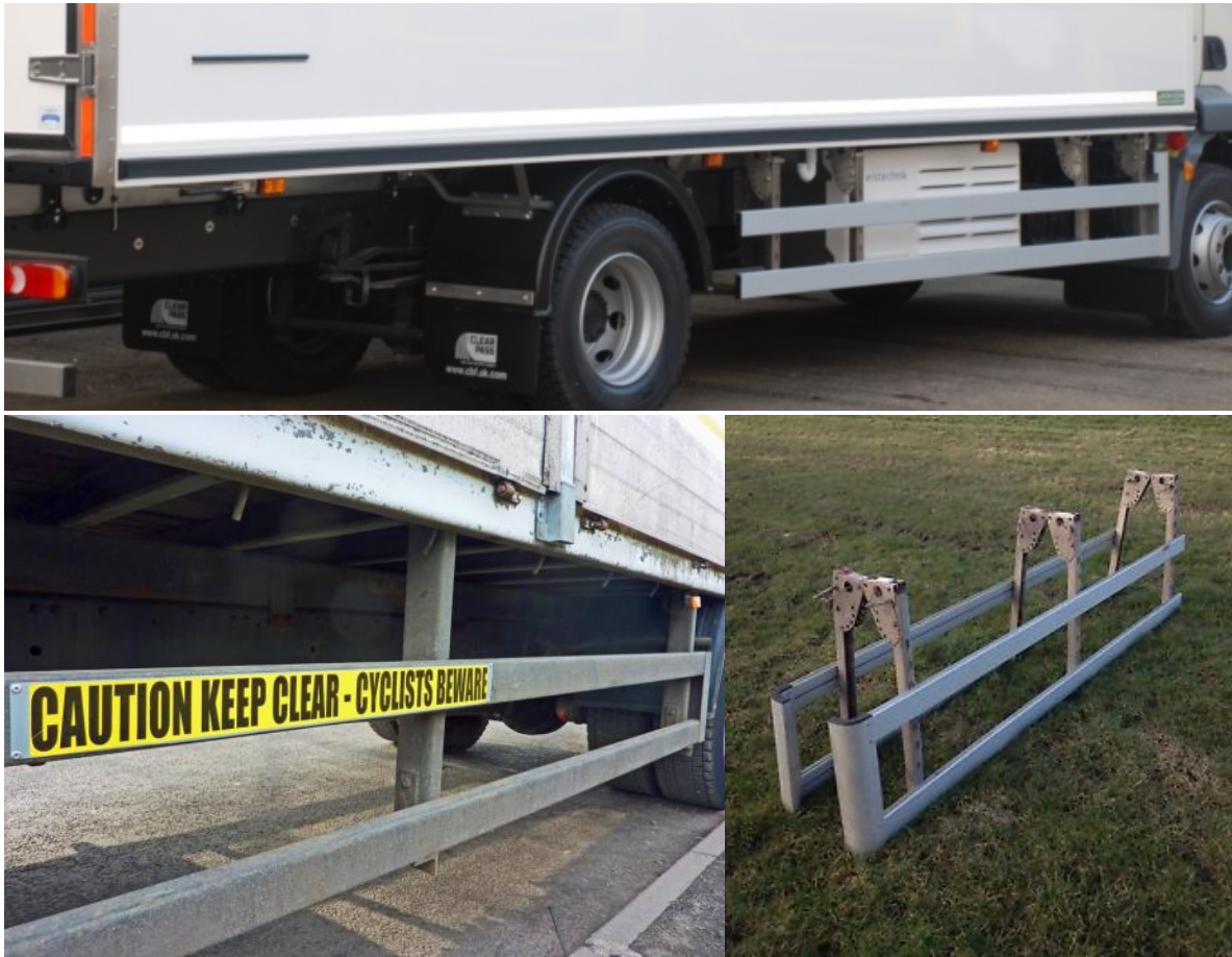
Figure 23. Retrofit sideguards mounted to underbody by vertical stanchions (UK), including around a refrigeration unit (top) and with conspicuous warning signage to bicyclists (bottom left). Bottom right: detached underbody-mounted sideguards.
