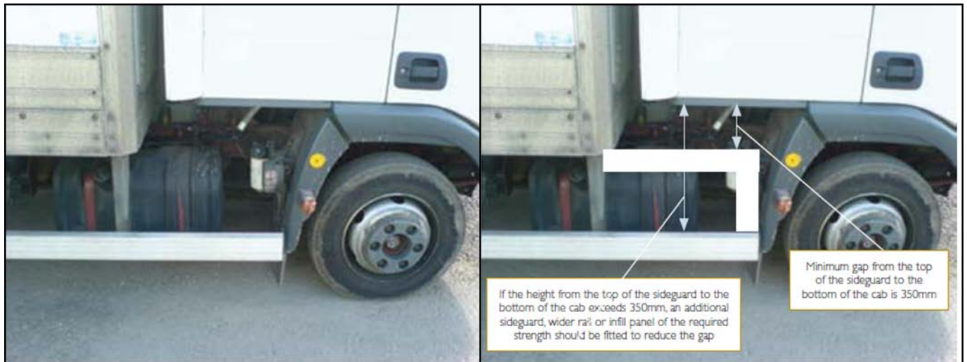
Figure 20. When the forward edge of the sideguard falls under the cab, any gap between the cab and the top of the sideguard exceeding 350 mm (13.8 in.) should be filled with an additional rail or panel of equal strength.
