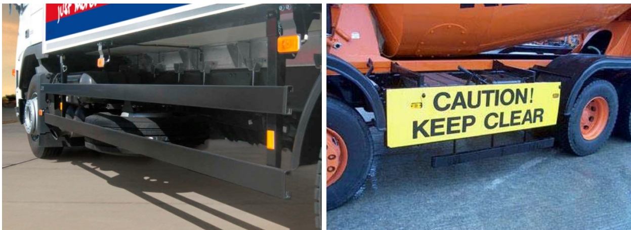
Figure 32. Sideguard accommodation of underbody spare wheel (left) and integration of reflectors/lights for conspicuity (left and right); integration of both a permanent upper and a flip-up lower sideguard that can be stowed for off-road access.
