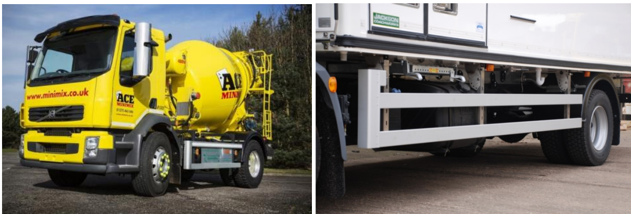
Figure 24. Sideguards on diesel particulate filter-equipped with Euro VI emissions standard compliant trucks, demonstrating compatibility of the two devices.
