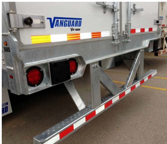
Figure 6. Rear impact guard, currently required on trailers by Federal Motor Vehicle Safety Standard 223.
