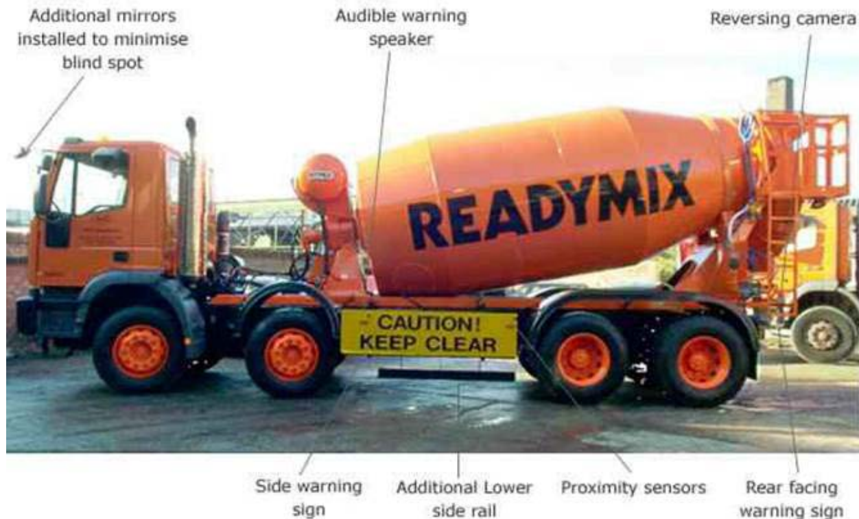
Figure 11. Panel sideguard on cement mixer with flip-up rail sideguard for city operation; also includes sensor and alarm (UK).
