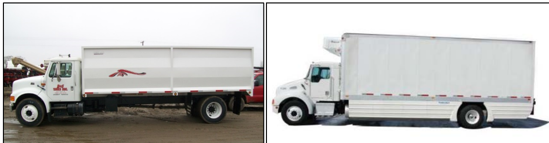
Figure 2. A large truck without sideguards (left) typically has an exposed space, often exceeding four feet in height, between the axles. During a crash with the truck, vulnerable road users can fall into the exposed space and suffer fatal crushing injuries. Sideguards (right) are designed to cover these exposed spaces.
