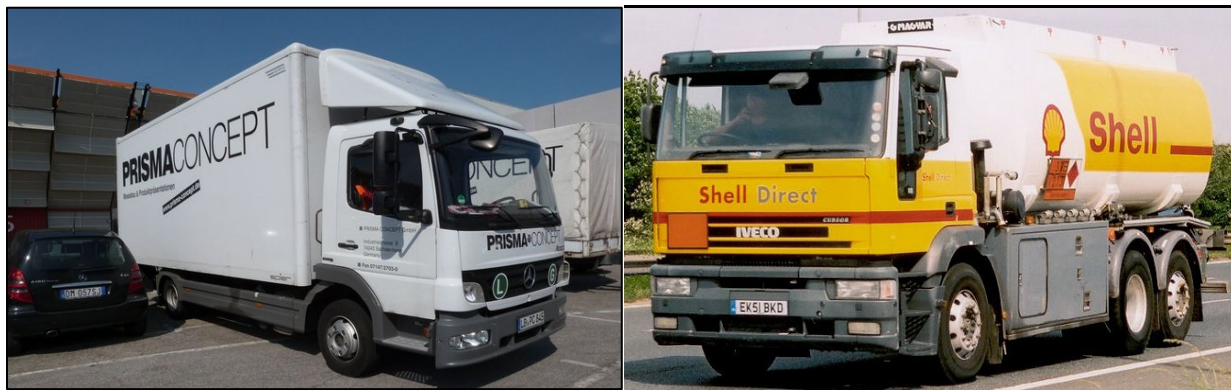
Figure 34. OEM integrated sideguards on single-unit trucks.
