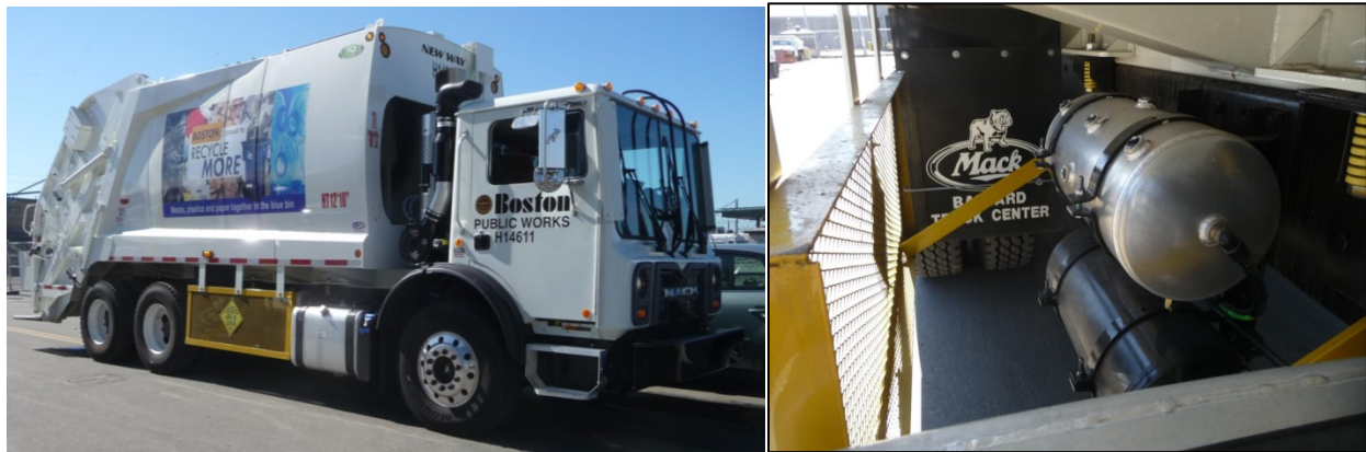
Figure 14. One of 19 retrofitted Boston Public Works collection trucks, with steel mesh sideguards mounted to both the body and the frame rail.
