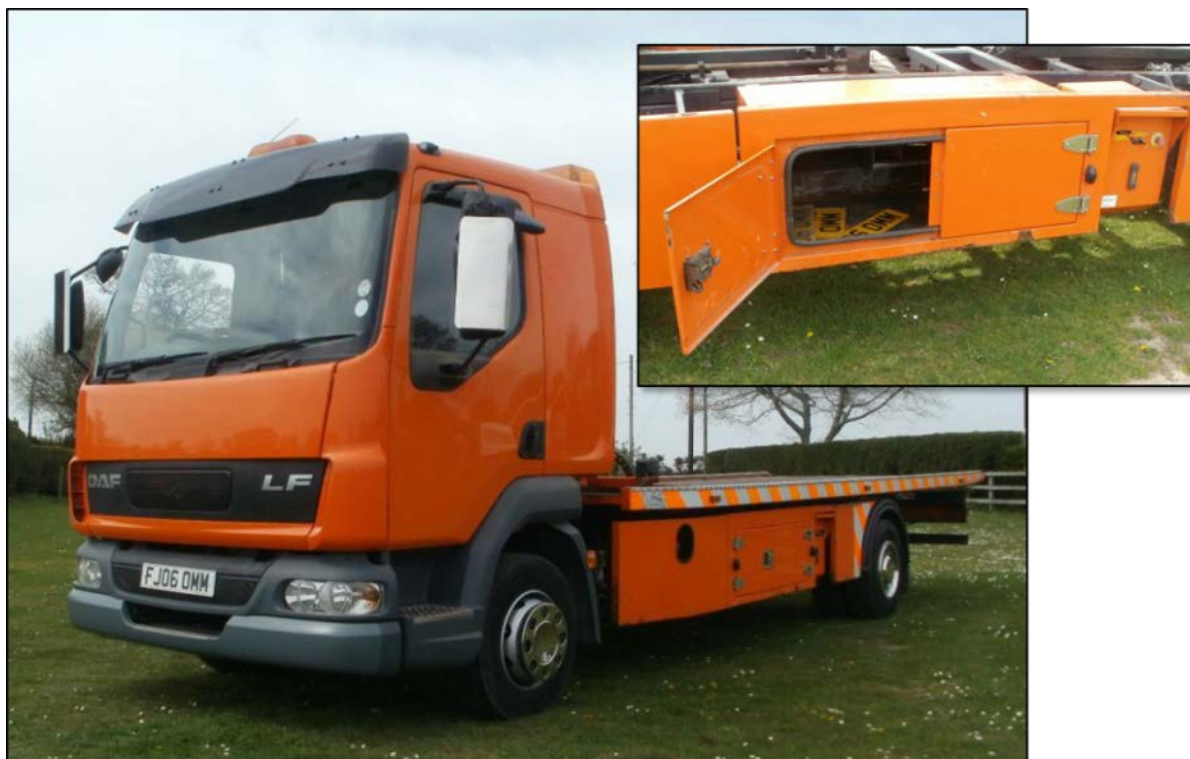
Figure 10. A panel-style sideguard with integrated toolboxes and hydraulic controls.
