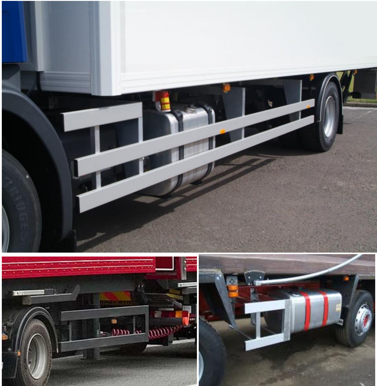
Figure 22. Sideguards installed around a fuel tanks (top and bottom right) and a stabilizer leg (bottom left). Each sideguard is mounted to the frame rails.
