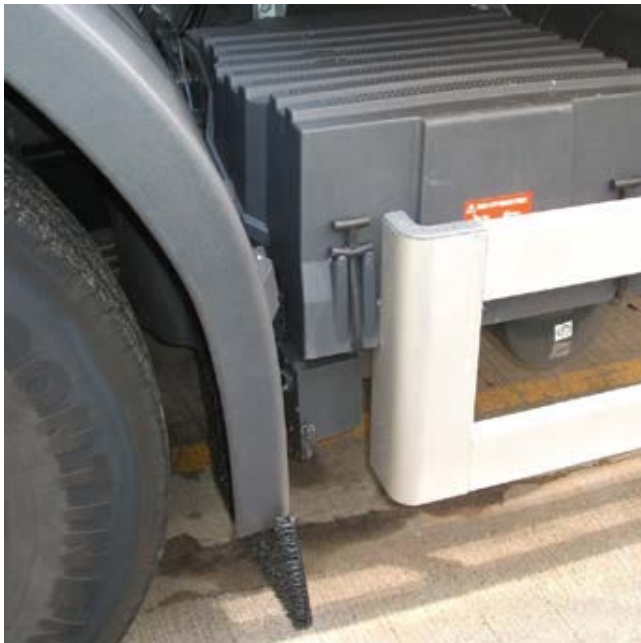
Figure 21. The forward edge of the sideguard should have a continuous surface that turns inwards for at least 100 mm (4 in.) This front continuous vertical outer surface and turn-in is optional when the front edge of the sideguard is within 100 mm (4 in.) of a permanent structure of the vehicle (vehicle cab/wheel arch).
