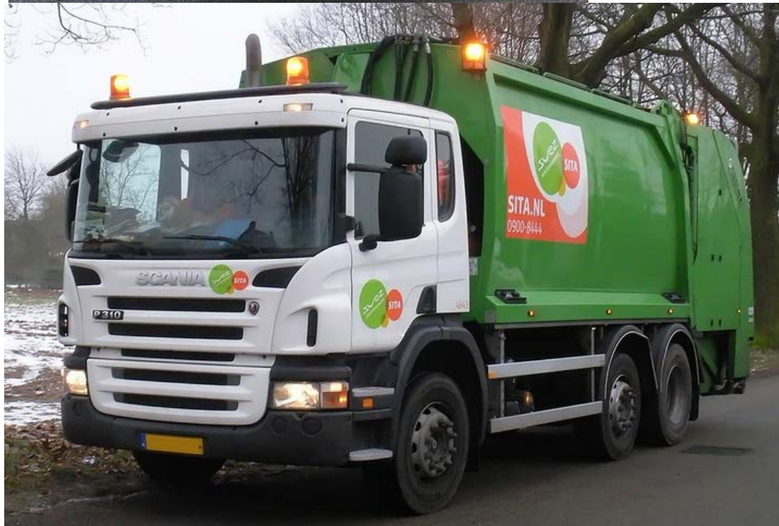
Figure 29. Rail-style sideguards on collection trucks.
