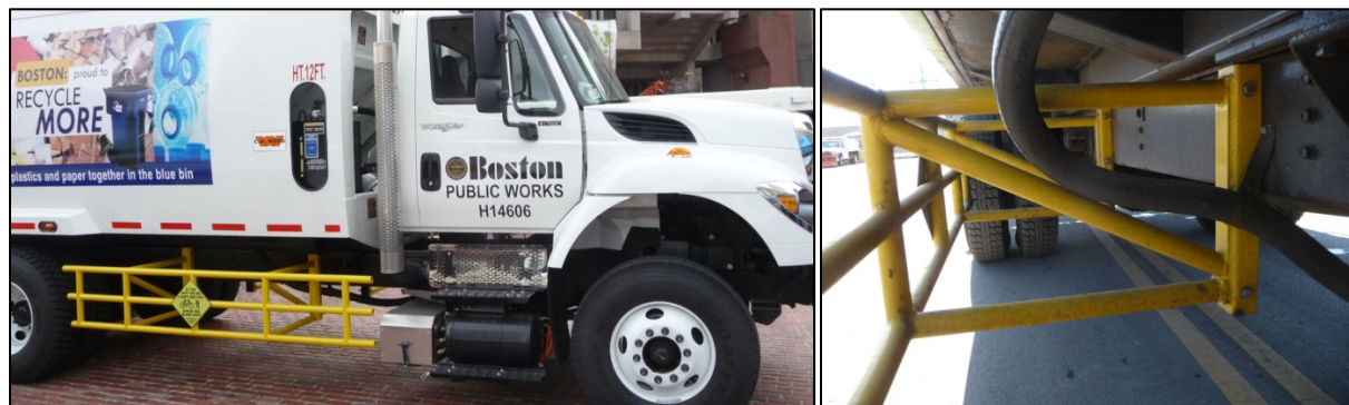
Figure 15. A Boston DPW collection truck with frame-mounted rail-style sideguards
