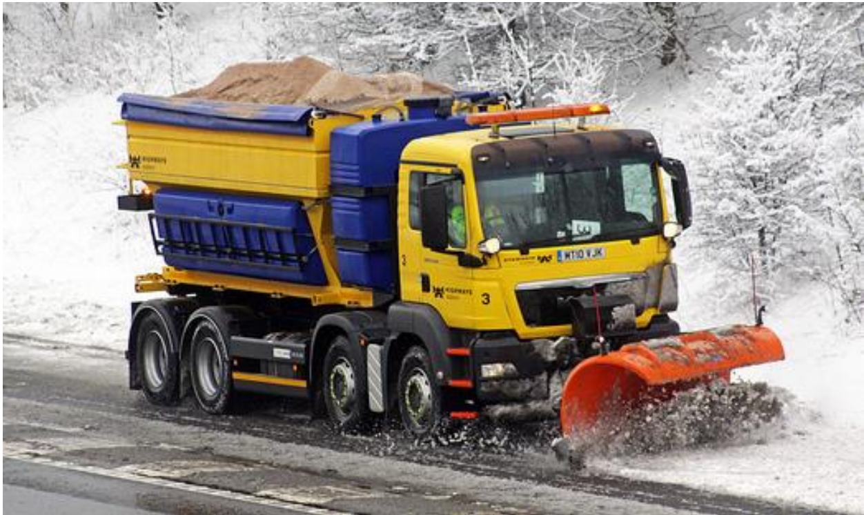
Figure 27. Panel-style sideguard on snow plow.
