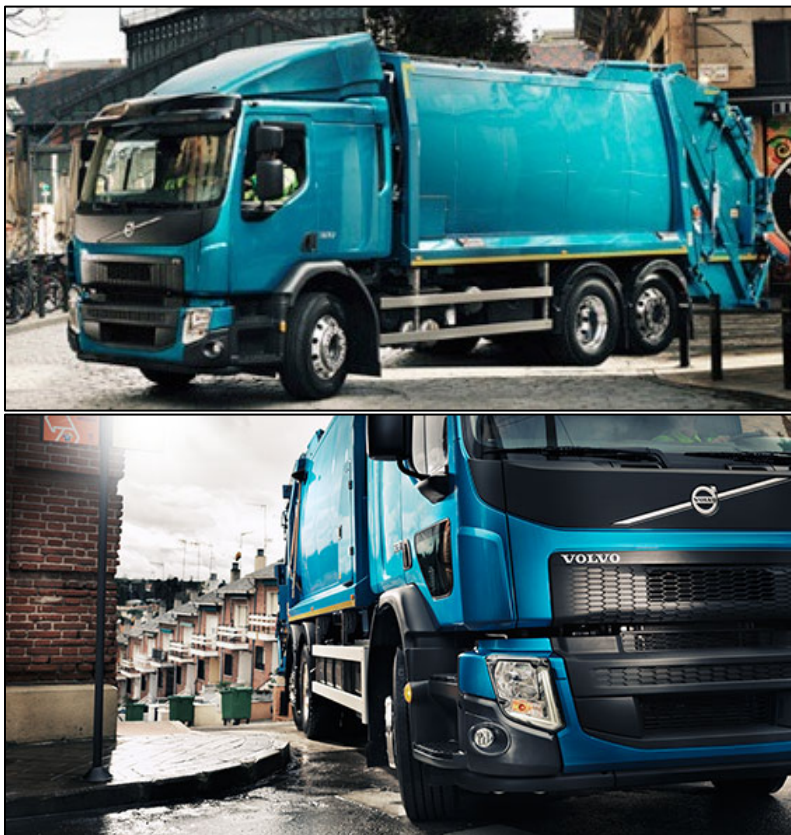
Figure 13. Mack/Volvo sideguard equipped collection vehicle currently manufactured for non-U.S. markets.
