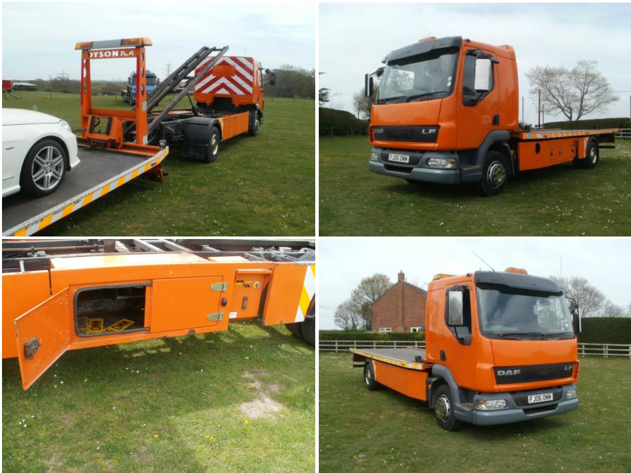
Figure 31. Panel-style sideguard with integrated toolboxes and control panel on UK roll-on-roll-off truck.
