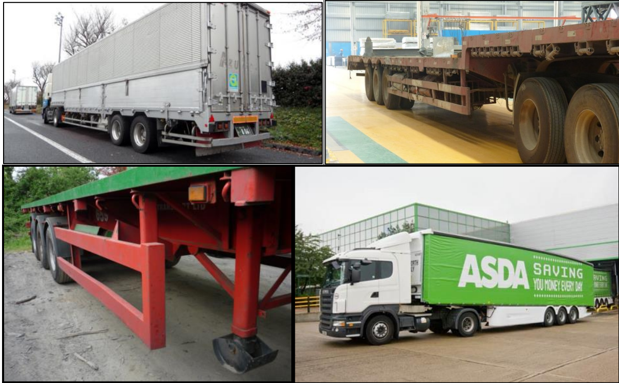
Figure 33. Rail-style trailer sideguards on Japanese (top left), Chinese (top right), and UK (bottom left) vehicles. Bottom right: OEM integrated panel-style sideguards on UK trailer.
