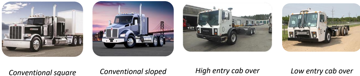
Figure 3: Truck cab types
