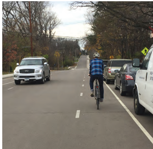
Figure 2.9 Advisory shoulders shown installed on a street with on-street parking. Source: FHWA.
