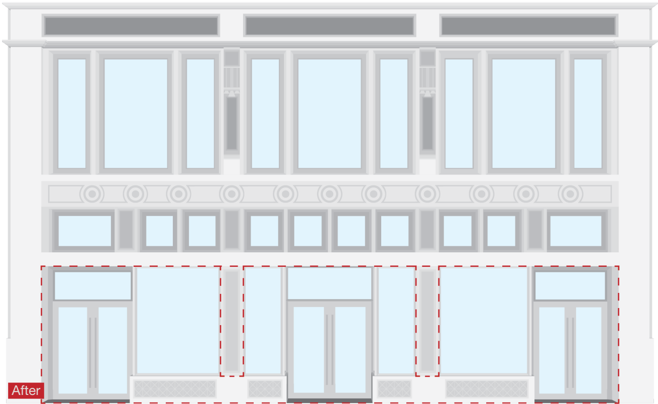
The new storefront recalls the original piers and restores the opening size.
