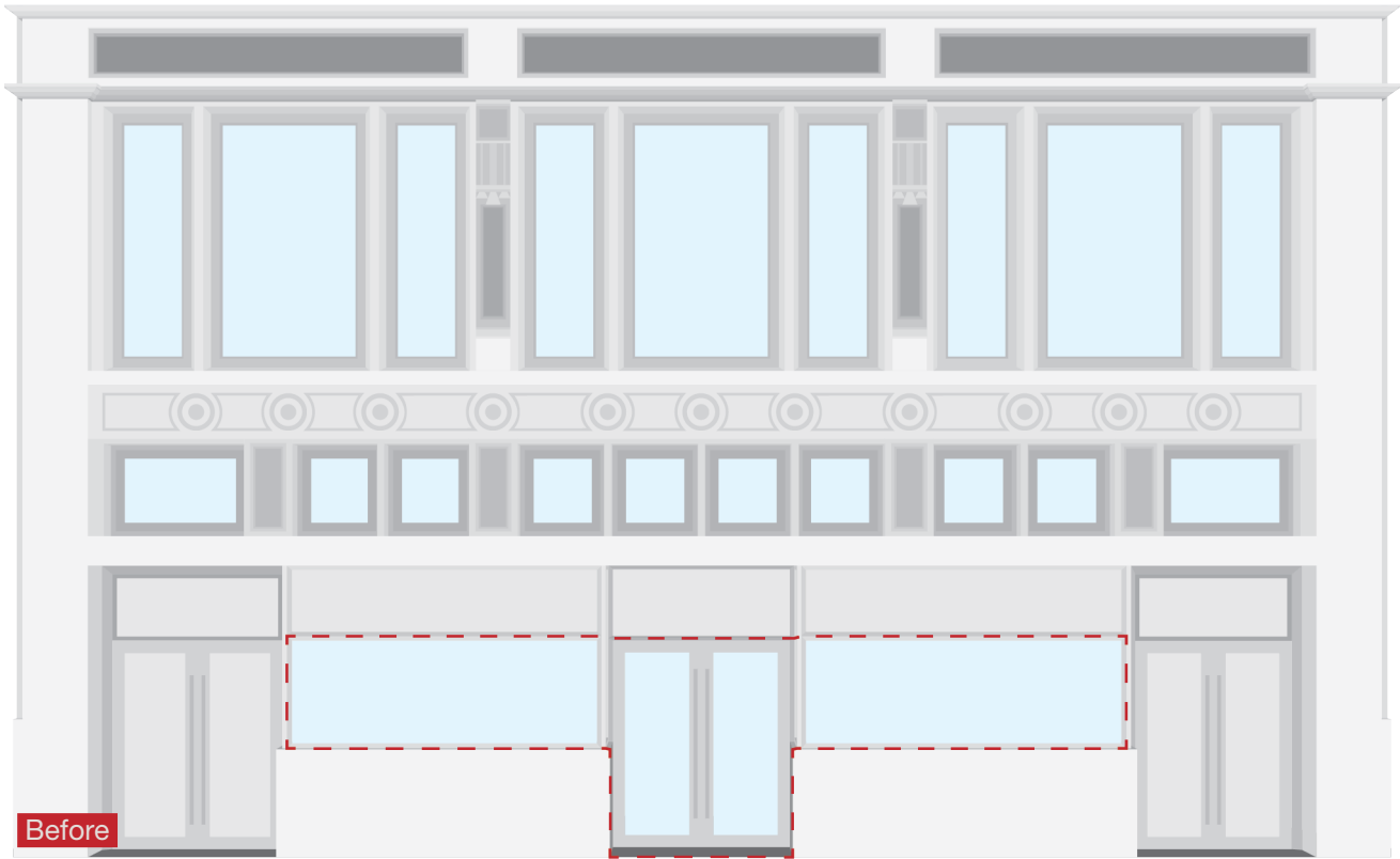
The original opening had been reduced in size and the piers had been removed.
