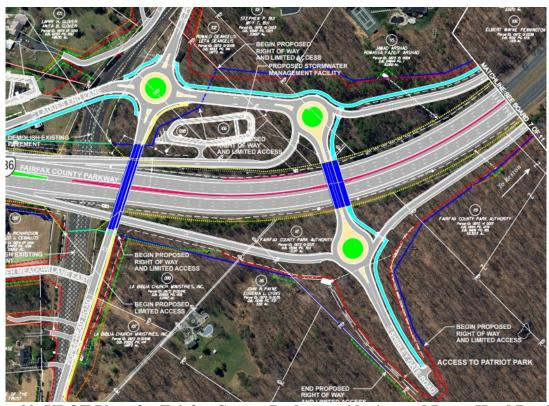
Figure 20: VDOT Plans for Fairfax County Parkway widening and Popes Head Road and Shirley Gate Road Extension Interchange
