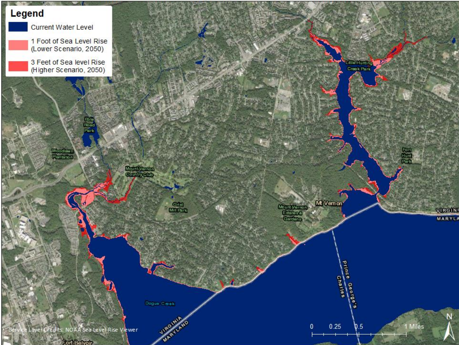
Figure 32: Projected Coastal Flooding due to Sea Level Rise for Mount Vernon Area between Dogue Creek and Little Hunting Creek
