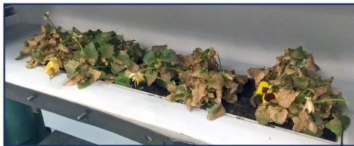
Plants after exposure to Ammonia in the CERT Chamber.
