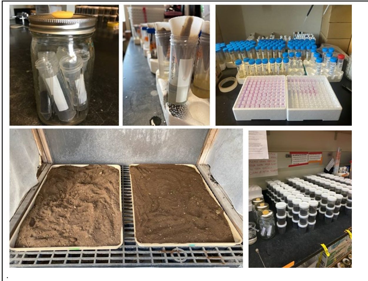
Figure 4.2. Aerobic incubation system followed by K_2SO_4 extraction and colorimetric analysis for nitrate and ammonium.
