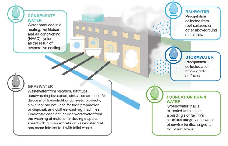
These onsite alternative water sources can be treated and reused to meet the following non-potable end uses:
