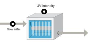
With the UV Intensity Setpoint approach, UVT monitoring is not required on the influent to the UV reactor. However, it is critical to consider the likely water quality of the influent in terms of UVT when selecting the appropriate reactor. An MBR-treated blackwater may have a UVT in the 60-75% range; if a reactor was validated only down to a UVT of 80%, the system will fail to meet the UV intensity setpoint and thus the reactor would not be an appropriate choice.
