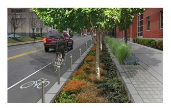
Figure 8: Low Impact Development Stormwater Management Techniques Incorporated into Street Design. This sort of design is encouraged in the McCormick Village Subarea.
