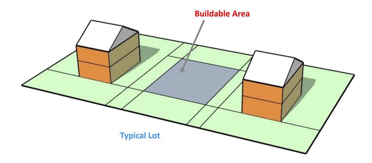
Example of buildable area for a triplex building on a typical lot
