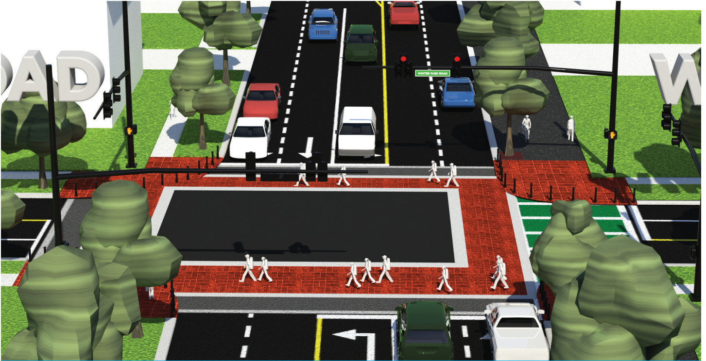
Raised intersection at Corrine Dr. & Winter Park Rd.
