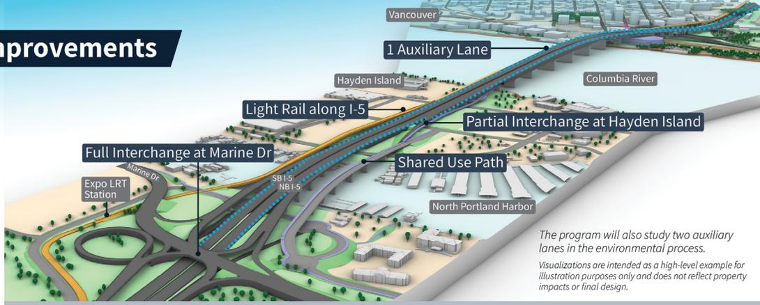
The program will also study two auxiliary lanes in the environmental process. Visualizations are intended as a high-level example for illustration purposes only and does not reflect property impacts or final design.
