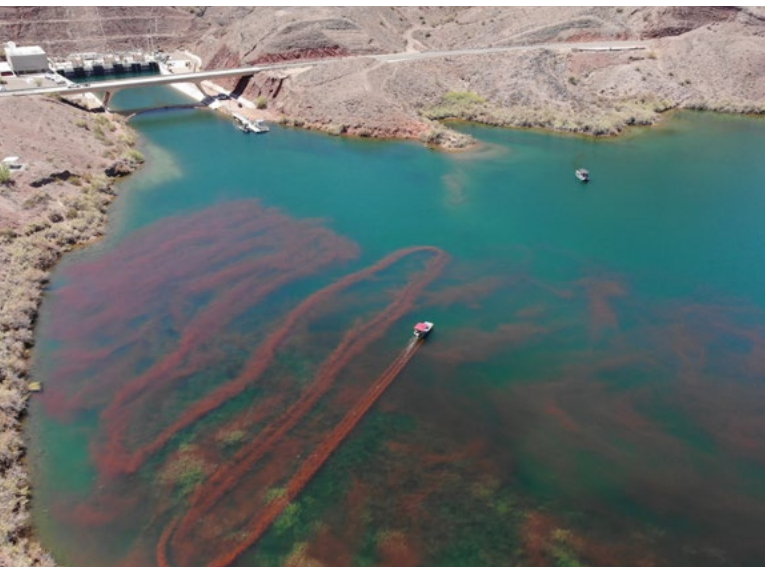
VEGETATION TREATMENT IN JUNE 2022. A DYE (RHODAMINE) WAS USED TO EVALUATE HERBICIDE COVERAGE AND DISTRIBUTION.
