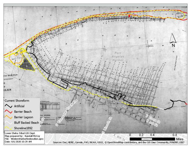
*Figure 3- Current Shoreline Conditions. Except for portions of Ediz hook, the entire shoreline is composed of fill with rock or sheet pile armoring. The Lagoon is reduced in size, and many areas are covered by over water structures, some of which are derelict.*
