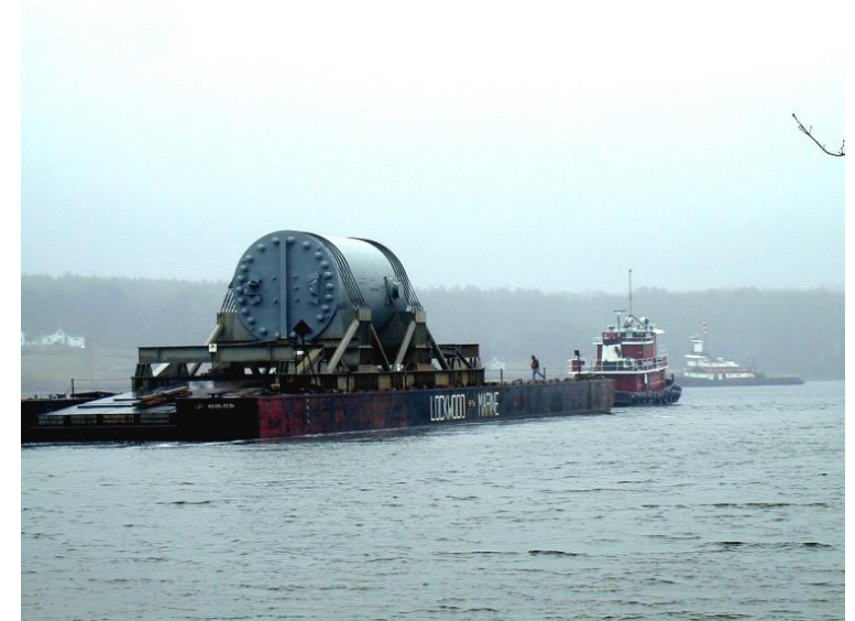
Reactor Pressure Vessel Shipping at Maine Yankee
