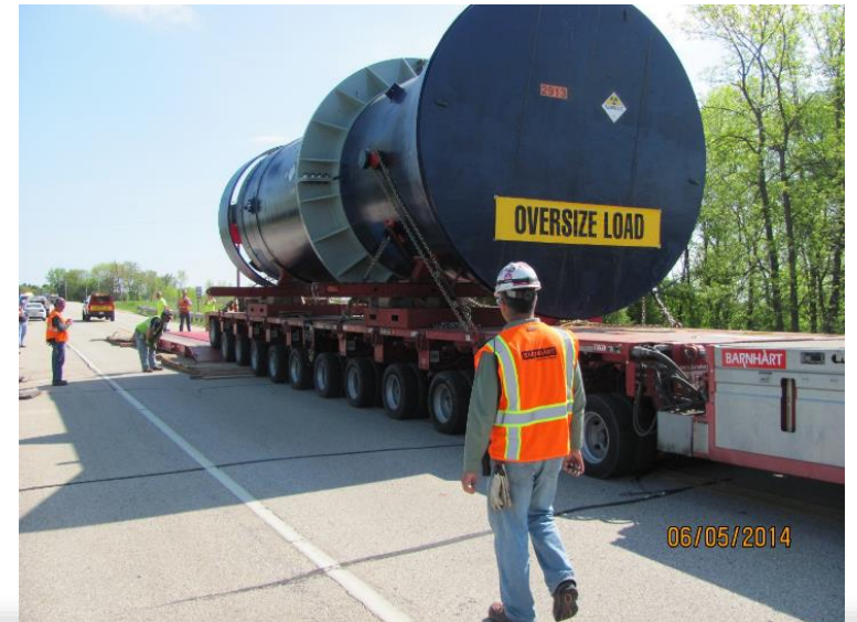
Reactor Pressure Vessel Shipping at La Crosse
