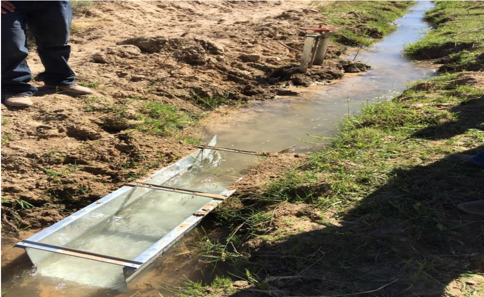
Figure 39. New flume and flow measurement device on irrigation diversion
