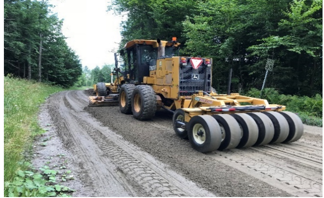
Figure 29. Operation of a grader-mounted compactor decreases erosion on gravel roads in the Town of Stowe. Equipment purchased through a DEC Clean Water Initiative Program grant. (Source: Town of Stowe)
