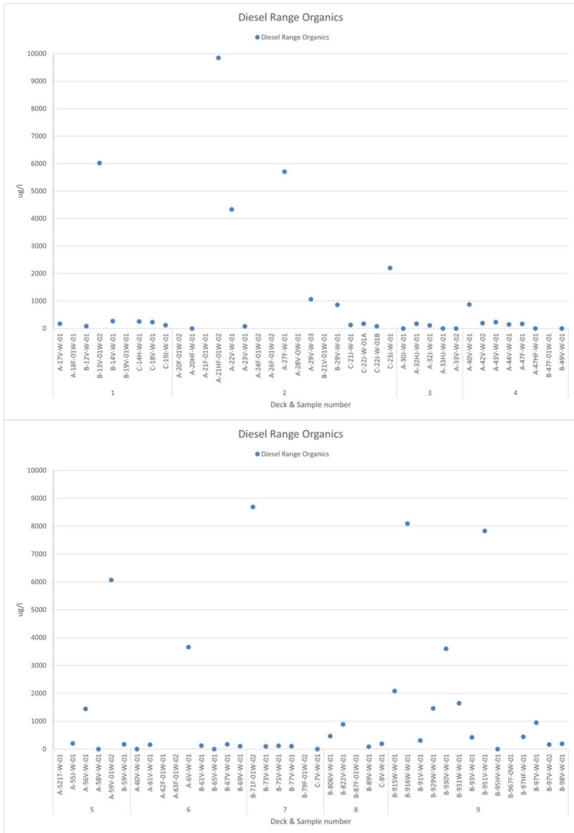
Figure 3-10. Concentration of diesel range organics in water on the USS Yorktown , for values up to 10,000 \mu\text{g/L} for decks 1-4 (top) and 5-9 (bottom), making lower values visible.
