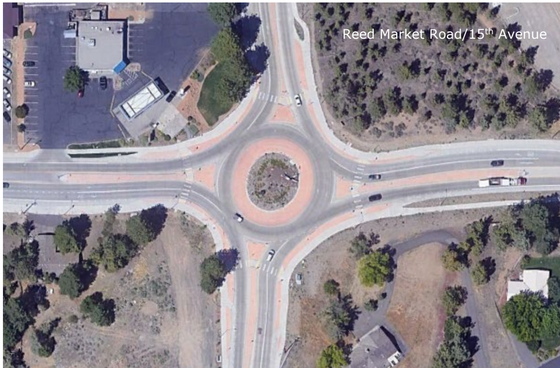
FIGURE 3: EXAMPLE OF PARTIAL DUAL-LANE ROUNDABOUT IN BEND
