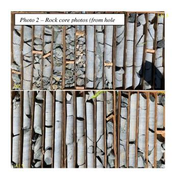
HQ sized core barrel. All three were drilled vertical. Total depths of the 3 holes were 360', 280' and 279' respectively. All were abandoned with grout.
