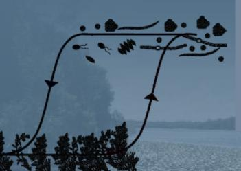
Concept of hysteresis where a clear shallow lake with weeds (macrophytes) is initially resilient to additional nutrient loading, but can rapidly transition into an algal-dominated system that requires additional measures to reduce nutrients and restore the clear-water state.
