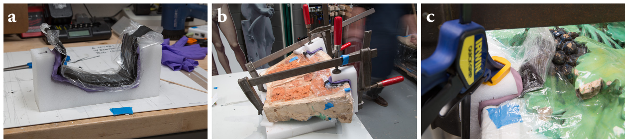
Fig. 15. (a) Layers of carbon fiber fabric and epoxy enclosed in plastic wrap package, laid into silicone inner mold. (b) Clamping while epoxy cures. (c) Detail showing clamping pressure on molds and carbon fiber. (Courtesy of C. Riccardelli, ©The Metropolitan Museum of Art)
