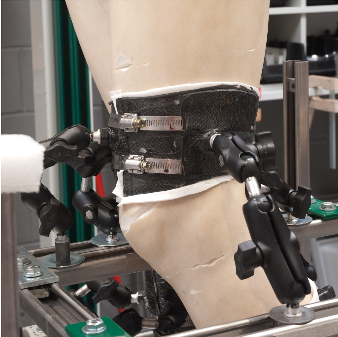
Fig. 8. Detail of Adam's left knee in the external armature. Hose clamps embedded into the carbon fiber layers allowed the strap to be tightened around the fragment or loosened to remove the strap at the end of the treatment; flange nuts in the strap allowed attachment of ball joints that connected to a rigid external framework. (Courtesy of C. Riccardelli, ©The Metropolitan Museum of Art)
