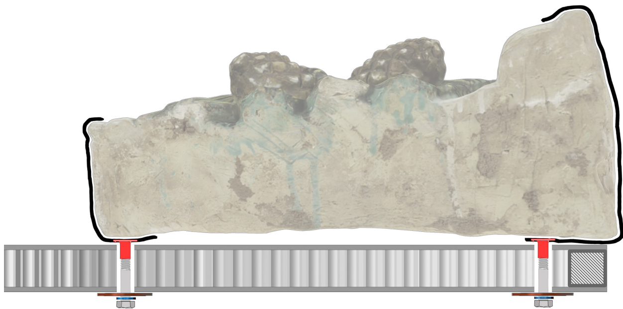
Fig. 10. Cross-sectional view of a garland section on the Prudence mounting system (Courtesy C. Riccardelli, ©The Metropolitan Museum of Art)
