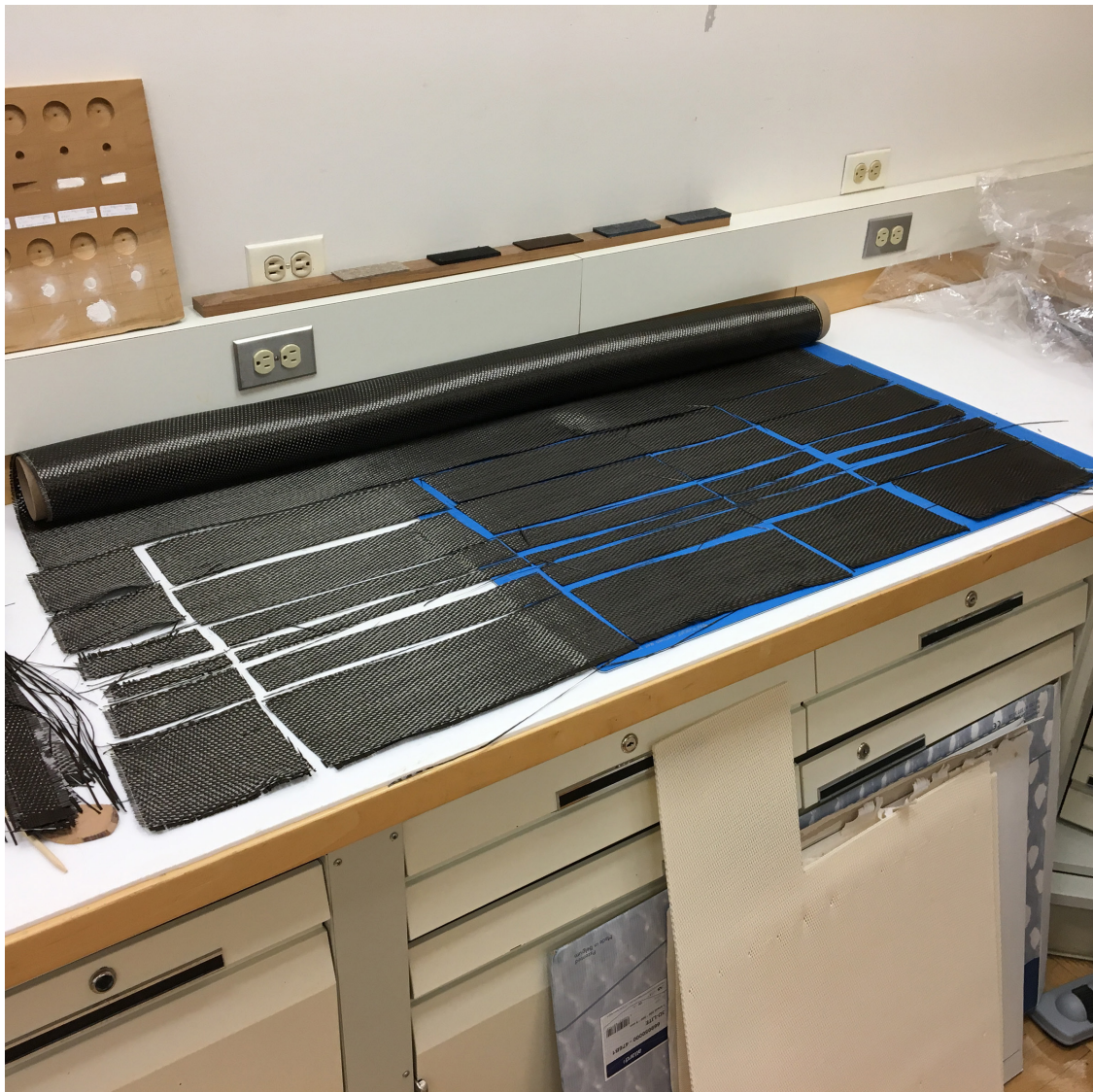
Fig. 12. Precutting the carbon fiber fabric into strips in preparation for layering with epoxy (Courtesy of D. Hausdorf, ©The Metropolitan Museum of Art)
