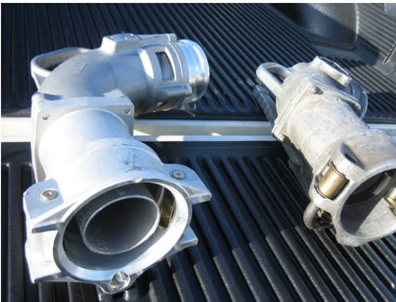
Figure 1. Two views of an elbow with a sleeve (left) and an elbow without (right)
