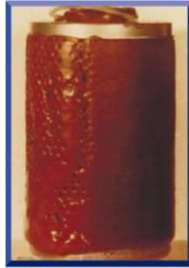
Fuel Filter Exposed to CFA Treated Fuel
