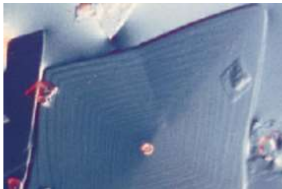
Figure 11 - Wax crystals in untreated diesel fuel [12]
